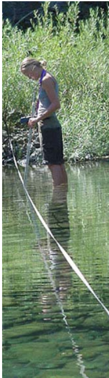
right, A measuring tape across the river guides where to read the flow levels on a meter.
